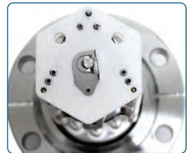
Field Replaceable Filament
