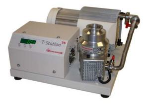
The T-Station comes with our new TAG (Turbo and Active Gauge) controller fitted as standard which enables single button start/stop of the system, the ability to control one of our Active Gauges<sup>\*</sup>, vent valve<sup>\*</sup> control and delayed start of the turbopump to either time or pressure if a gauge is fitted, making the T-Station ideal for general laboratory needs.
